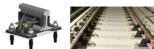
Example of Rail Fastening System with Pad to Minimize Vibration (Pandrol Vanguard Type)
